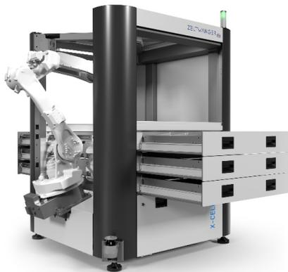
Up to four gripper change systems can be integrated in the X-CELL WB. This means that multiple orders can be processed automatically without the operator having to change the gripper. An integrated reversible gripper enables machining of the sixth side without manual reclamping. The single, double, and special grippers are all equipped with an integrated blowing nozzle and position monitoring for component recognition.
