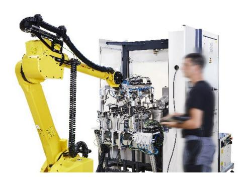
The X-LOAD eco handling cell from ZELTWANGER, which has been adapted to customer requirements, enables efficient and precise assembly of insert moulding inserts.
